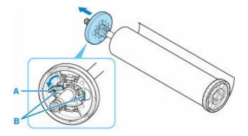
**11.** Remove printed material that has been taken up, from roll holder for each paper core.
