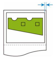
If the lower roll of paper has smaller margins than the upper roll of paper, from which the paper has been fed, then paper is switched automatically, and the image is printed on the lower roll paper.
