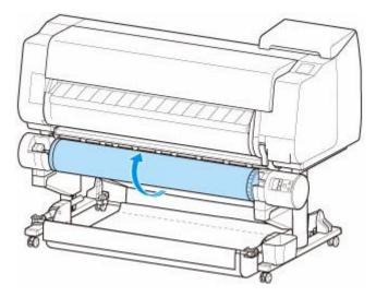
Apply adhesive tape to the rewound paper to hold it in place, if necessary.
