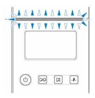
If the **Status** lamp is flashing orange, check the message on the touch screen and take action as necessary.
