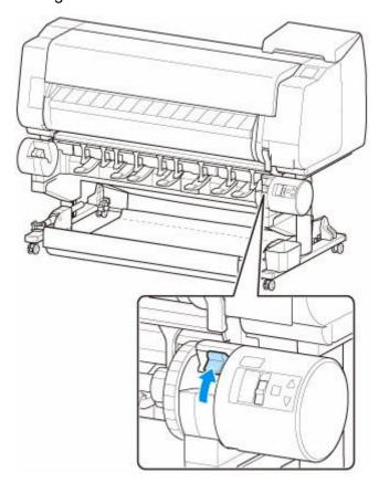
**3.** Hold flanges (A) so that holder stopper is on left, align roll holder shaft with roll holder slot left and right guide grooves (B), and load.
