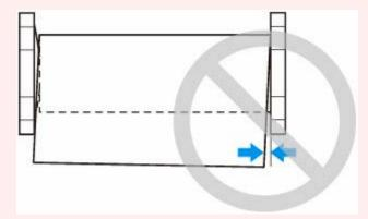
Depending on the paper, the roll paper may be scratched when being fed and not feed well.
