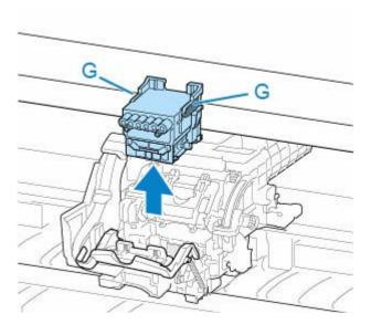
• Never touch the metal contacts of the carriage. Furthermore, do not allow any dirt or debris to become adhered to the metal contacts of the carriage. These may damage the printer.
