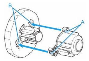
**5.** Insert holder stopper from left into roll holder as shown, and then while holding in position (B), push firmly until holder stopper flange (A) touches roll paper. Lock the holder stopper lever (C) by rotating it towards .
