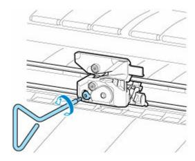
7. Remove cutter blade while holding D.
