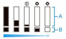
If the touch screen indicates to replace the ink tank, replace the ink tank. If a message is displayed indicating to check the remaining ink levels, or after tasks that consume a lot of ink such as large-format printing or head cleaning, check the remaining levels and replace ink tank as needed.
