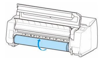
7. Hold Roll Holder by its flanges (A) and remove from roll holder slot.
