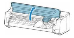
**3.** If the Carriage is out, move the Carriage to the left or right side, away from the jammed paper.
