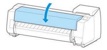
**5.** Tape down printer covers to secure them, in the reverse order of tape removal during installation.
