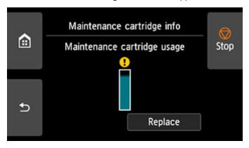
If the touch screen indicates to replace the maintenance cartridge, replace the maintenance cartridge.
