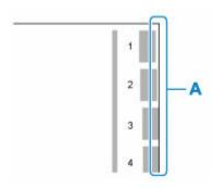
Check the paper edge (A) of the 1st to 8th on the output pattern and select the number that has the appropriate amount of extension.
