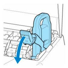
**3.** Push ink tank lock lever firmly down until it does not return.
