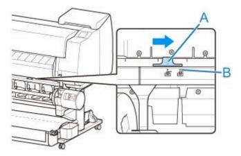
**10.** Change **Inward/Outward Winding Changeover** switch on roll unit to desired winding direction.
