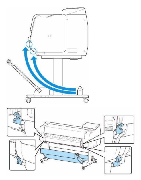
• When attaching the basket rod (cord side) to the front of the printer, make sure both ends of the rod (A) are securely hooked onto the attachment parts.
