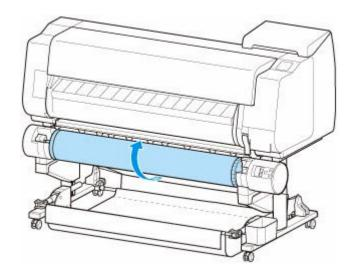
**6.** Change **Roll Holder Lock** switch on roll unit to release position.
