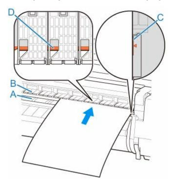
When you insert the sheet, it will adhere automatically to the surface of the platen.
