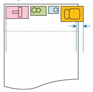
If an image is running off the edge of the paper as shown above, the subsequent images are printed on the next sheet.
