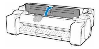
**6.** Align the angle adjustment lever with the red square and close the top cover.
