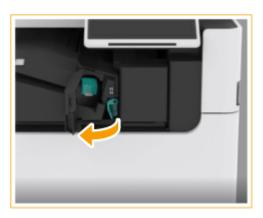
**4** Hold the lever ( **6**), and slide the inner finisher to the left.
