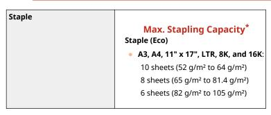
\* When the standard staple cartridge is attached. (The maximum stapling capacity may vary, depending on the paper type and weight.)
