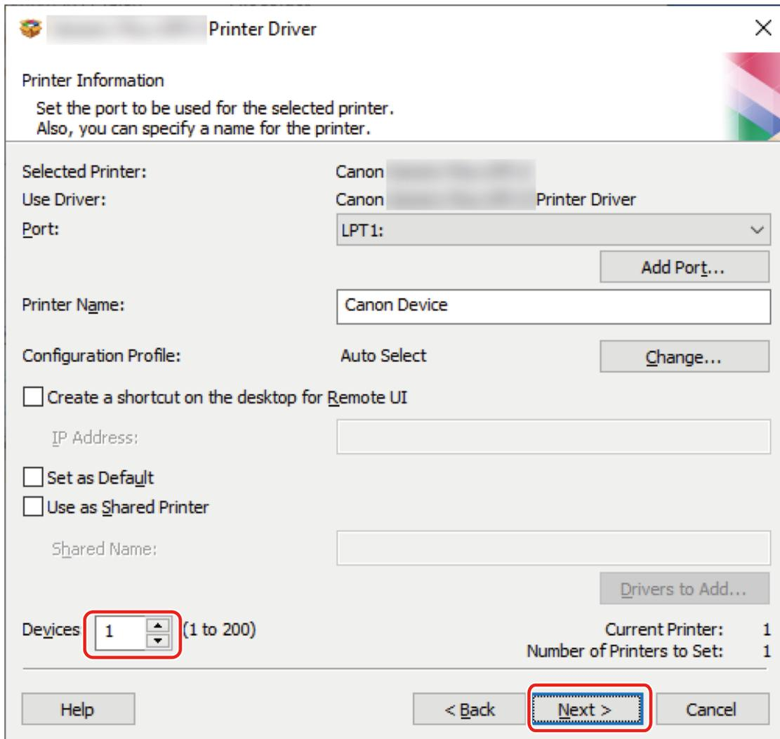
If multiple configuration profiles were selected in step 6.(P. 29) , or multiple devices were specified in [Devices], the [Printer Information] screen is repeatedly displayed the number of times corresponding to [Number of Printers to Set]. Repeat steps 7.(P. 30) to 9.(P. 32) for each device.
