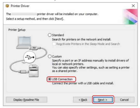
6 When the following screen appears, connect the device and computer with a USB cable → turn on the device.
