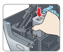
Close and press the round, indented portion on the Clear Ink Tank Locking Cover until it snaps firmly into place, locking the ink tank.
