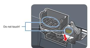
5 Push the Print Head to hold it in place, and lower the Print Head Lock Lever.
