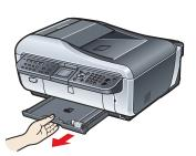
2 Load four sheets of plain paper in the Cassette with the printing side facing DOWN and the leading edge to the far side, align the paper stack against the right side of the Cassette, then slide the Paper Guides to fit to the loaded paper stack.
