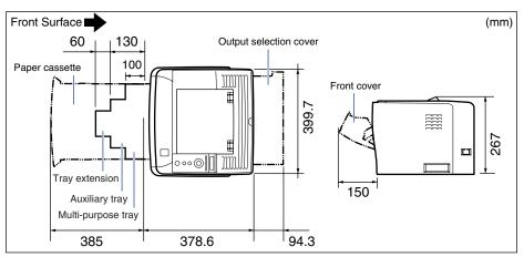
State with the paper feeder installed
