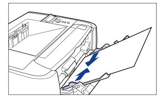
Be sure to align the paper guides with the width of the paper. If the paper guides are too loose or too tight, this may result in misfeeds or paper jams.
