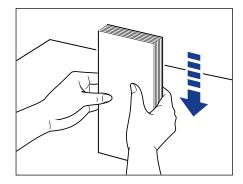
**8** Gently load the stack of envelopes with the address side facing up until it touches the back of the tray.
