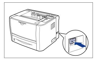
The indicators and display on the control panel come on, and the printer initiates a self-diagnostic test on the printer unit and optional accessories.
