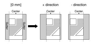
Specify on which edge of the paper, the long edge or short edge, the gutter is to be created in BIND.LOCATION (See the previous item). On which edge (top/ bottom/left/right) of the paper the gutter is created depends on the setting for BIND.LOCATION and which value "+" or "-" is specified for this item.
