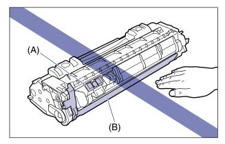
**9** Remove the packing material with paper inside the front cover.
