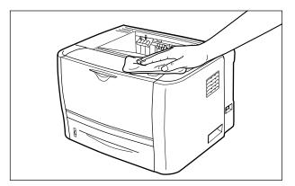
**4** After wiping off the dirt, wipe the printer with a dry cloth.
