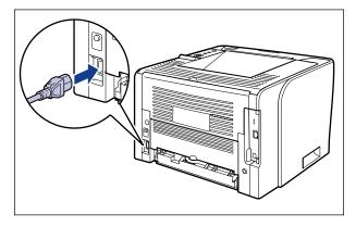
**3** Plug the power plug into the AC power outlet.
