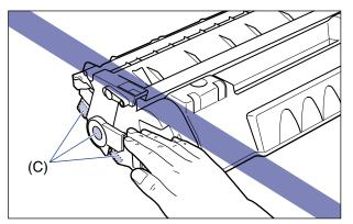
• When handling a toner cartridge, hold it properly as shown in the figure and handle it with the arrowed side facing up. Do not place it vertically or upside-down.
