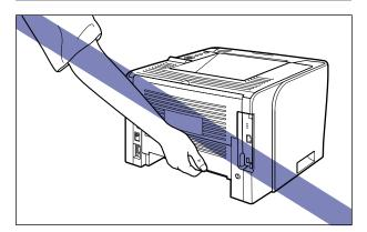
• The back portion (A) of the printer is relatively heavy. Be careful not to get off-balanced when lifting the printer. If you do so, you may drop the printer, resulting in personal injury.
