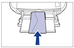
• When loading envelopes of the Envelope B5 size, close the flaps and load them so that the envelopes are fed from the top (the edge with the flap).
