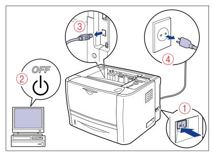
**2** Remove all the interface cables and the power cord from the printer.
