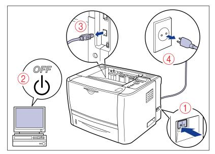
**2** Remove all the interface cables and the power cord from the printer.
