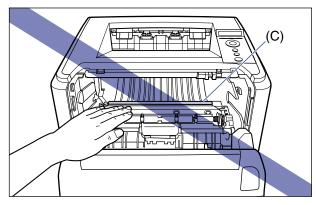
• The face-down output tray and its surroundings become hot during or immediately after using the printer. Do not touch the face-down output tray and its surroundings when removing the jammed paper or performing the related operation.
