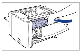
Immediately place the removed toner cartridge into the original protective bag or wrap it with a thick cloth.
