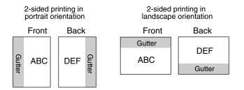
If SHORT EDGE is specified, the binding location is created on the short edge of the paper.
