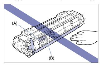
9 Hold the toner cartridge properly with the arrowed side facing up as shown in the figure.
