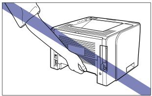
• The rear portion (A) of the printer is relatively heavy. Be careful not to become off-balance when lifting the printer. If you do so, you may drop the printer, resulting in personal injury.
