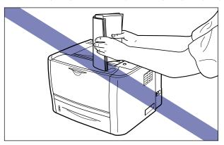
Do not open the covers on the printer during printing. This may result in damage to the printer.
