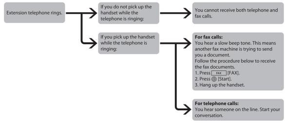
\*If <REMOTE RX> is set to <ON>, you can also start to receive fax documents by dialing from your telephone. (See "Receiving Documents Manually with an External Telephone (Remote RX)," on p. 5-36.)
