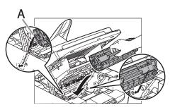
Align the guide (A) on the left side of the toner cartridge with the groove inside the machine.
