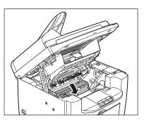
4 Close the printer cover and lower the scanning platform.
