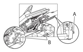
Push down the toner cartridge to make sure it is properly set in the machine.
