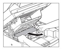
Gently pull the jammed paper between the fixing assembly (A) and transfer roller (B) until the leading edge emerges from the machine.
