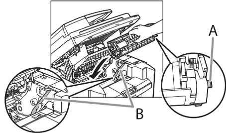
**10** Push the toner cartridge to make sure it is properly set in the machine.
