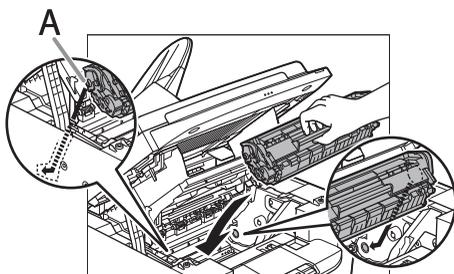
Align the guide (A) on the left side of the toner cartridge with the groove inside the machine.
