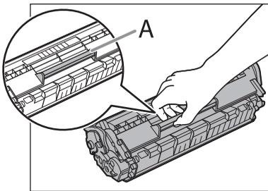
**9** Insert the toner cartridge so that the protrusion (A) on the right side of the toner cartridge fits into the guide (B) located on the right side of the machine and slide it down parallel to the guide.
