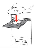
Turn on the computer, then insert the **Setup CD-ROM** into the CD-ROM drive.
