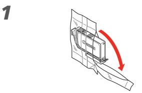
Remove the ink tank from its package.
