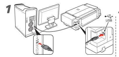
Connect the printer to the computer with a USB cable.
