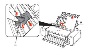
When the **Print Head Alignment** screen appears, load two sheets of A4 or Letter-sized plain paper in the Rear Tray (A) as shown.
