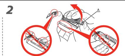
Remove and discard the orange protective cap (A) located on the bottom of the ink tank.
