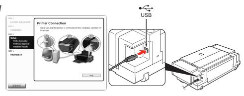
When the **Printer Connection** screen appears, connect the printer to the computer with a USB cable.
