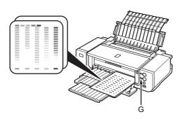
Make sure that the pattern shown is printed, then click **Next** on the **Print Head Alignment** screen.
