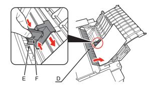
Pinch and slide the Paper Guide (E) against the left edge of the paper, then close the Feed Slot Cover (D).
