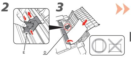
Open the Feed Slot Cover (D), then pinch and slide the Paper Guide (E).
