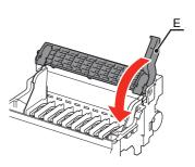
Lower the Print Head Lock Lever (E) completely.
