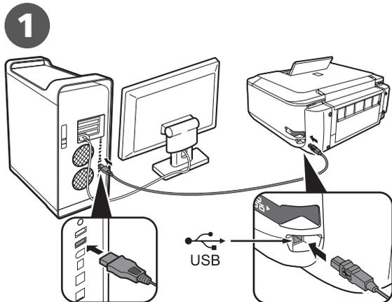
Connect one end of the USB cable to the computer and the other to the machine. Make sure the machine is turned on.
