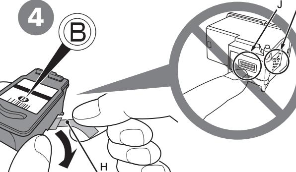
Pull the orange protective tape (H) in the direction of the arrow and remove it gently.
