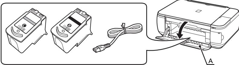
The FINE Cartridges and power code are placed inside of the Paper Output Tray (A). Open the Paper Output Tray, and take out them.
