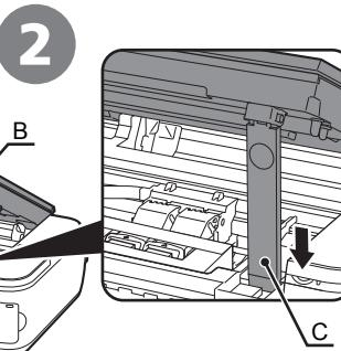
Lift the Scanning Unit (Cover) (B) and fix it with the Scanning Unit Support (C).
