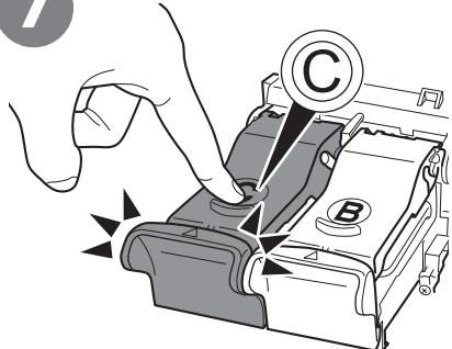
Insert the Color FINE Cartridge © into the left FINE Cartridge Holder © in the same way as ®.
