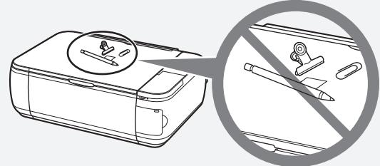
Do not install the machine where an object may fall on it. The object may fall inside the machine, resulting in malfunction.
