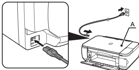
Plug the power cord into the left side of the machine, then connect the other end to the wall outlet.
