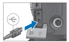
Connect the plug with the < → > mark facing the front of the camera.
