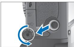
Attach the cap on the fixing screw.
