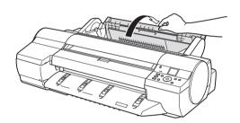
Hold the flange (a) of the roll holder and align its axis with the left and right guide grooves (b) in the roll holder slots. Make sure that the colors of the guide grooves and the roll holder axis are the same before loading the paper.
