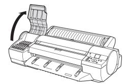
While pressing the stopper of the ink tank lock lever inwards, open the ink tank lock lever upwards.
