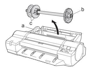
Remove the orange tape on the top cover (a) and the ejection guide (b) and all the packing materials.
