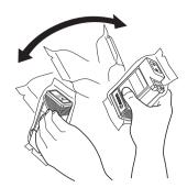
• Failure to shake the ink tanks may result in reduced print quality because ink ingredients have settled on the bottom of the tank.
