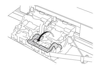
Lift the printhead fixer cover to open it fully.
