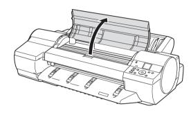
Pull the printhead fixer lever forward all the way to open it completely.
