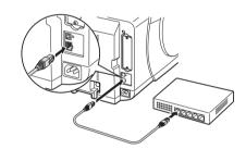
If the printer is on, the Link indicator under the LAN port lights. 1000Base-T The top and bottom LEDs light. connection The LED on the bottom 100Base-TX connection lights green. The LED on the top lights 10Base-T connection orange.
