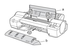
Lift the belt stopper (b) from the carriage shaft (a) and pull it towards you to remove
