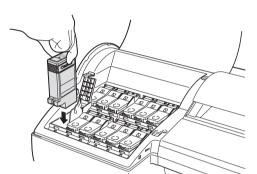
• If the ink tank does not fit in the holder, make sure the color of the ink tank lock lever matches the color of the ink tank, and check the orientation of the ink
