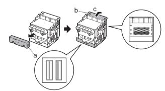
• Never touch the parts covered by the protective parts. Doing so may damage the printhead and affect printing quality.
