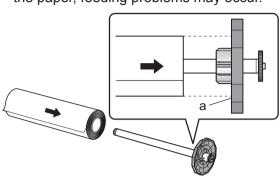
Slide the holder stopper for the 2-inch paper core onto the roll holder from the left until its flange (a) is against the roll of paper.
