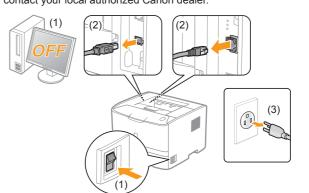
When installing or removing the optional accessories, be sure to turn the printer OFF, unplug the power plug, and then disconnect all the interface cables and power cord from the printer. Otherwise, the power cord or interface cables may be damaged, resulting in a fire or electrical shock.
