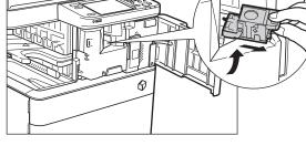
**3** Press the area indicated by PUSH, and then lift up the staple cartridge.
