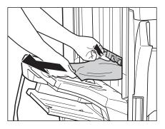
If you are using the Staple Finisher-A1, open the guide (F-B3), and remove any jammed paper.
