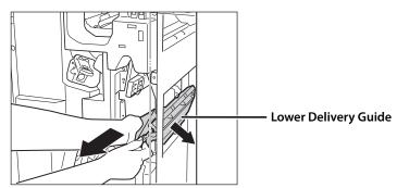
**4** Tilt the lower delivery guide to the right, and remove any jammed paper.
