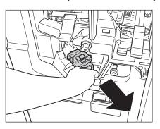
3 Turn over the staple case, and open the cover while pressing PUSH on both sides of the staple case.
