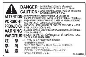
This machine has been classified under IEC60825-1:2007 and EN60825-1: 2007 and conforms to the following classes:
