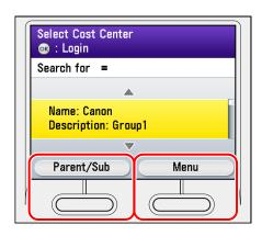
Enter your PIN code (up to 20) digits) using (0) - (9) (numeric keys) → press the right Any key to select <Log In>.
