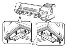
Mount the printer on the assembled **Stand** and tighten the screws firmly.
