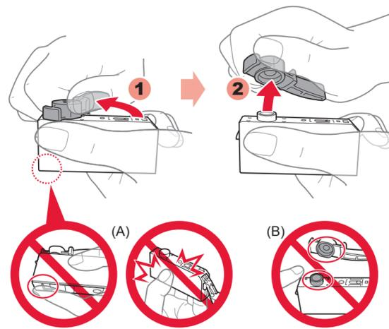
3 Twist and remove the orange cap.
