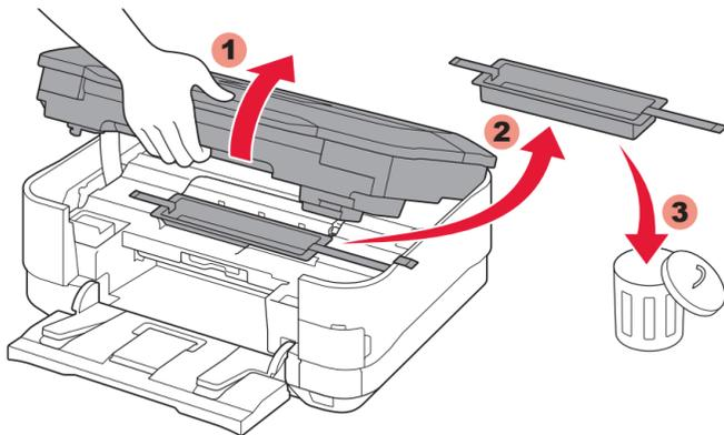
3 Lift the Scanning Unit / Cover, then remove the orange tape and protective material.
