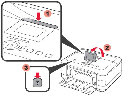
6 Adjust the angle of the LCD, then press the **ON** button.
