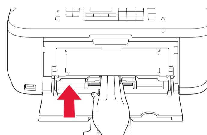
Insert paper with the printable side down until it stops. When using photo paper, machine settings for media type and size should be adjusted. For details, refer to the **On-screen Manual** which will be installed later.
