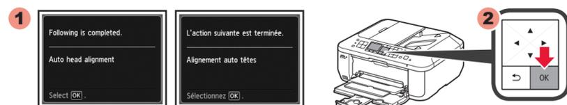
10 When the screen as shown is displayed, press the OK button to complete Print Head Alignment.
