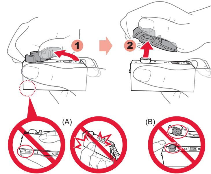
3 Twist and remove the orange cap.
