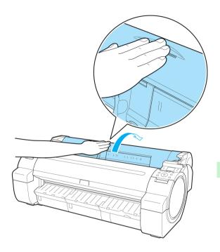
Holding the Roll Holder flange (a), rest the Roll Holder shaft on the Roll Ledge (b). At this time, position the holder so that the **R** label (c) on the [W label (c) on the Roll Holder flange is aligned with the **R** label (d) on the printer .
