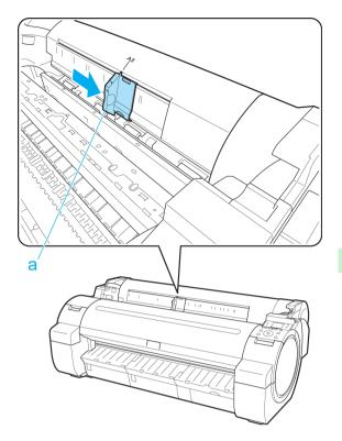
Load a single sheet printing-side up in the Paper Feed Slot, with the right edge aligned with the Paper Alignment Guide (a) to the right of the Roll Cover.
