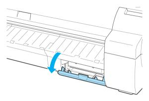
Hold the used Maintenance Cartridge by the grip (a) with one hand and put your other hand under the Maintenance Cartridge to hold it firmly on the bottom, keeping it level as you pull it out.
