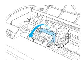
Pull up the Printhead Fixer Cover to open it complete-
