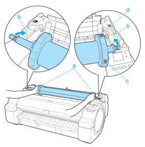
Holding the Roll Holder flange (a), guide the holder along the Roll Loading Slots (b) on both ends, keeping the holder level as you load it in the Roll Holder Slot.
