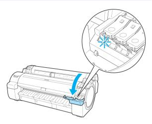
Press the tip of the Ink Tank Lock Lever of the color for replacement horizontally and pull the Ink Tank Lock Lever up to open it.
