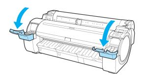
Pressing the tip of the lnk Tank Lock Lever horizontally, lift the lnk Tank Lock Lever to release the lock.
