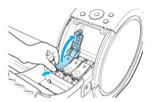
Hold the Ink Tank by the grips and remove it. Press the **OK** button.
