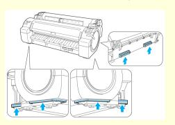
Remove tape and packaging material attached to the printer.
