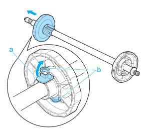
2 Insert the respective attachments for the roll paper core on the Roll Holder and Holder Stopper.
