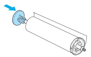
Load the roll Roll Media in the printer.
