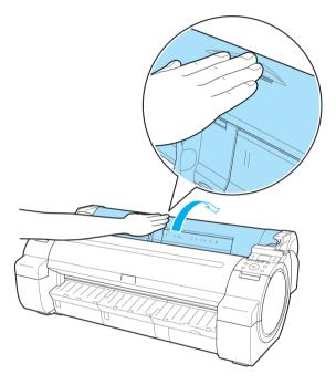
6 Using both hands, rotate the Roll Holder toward the back to rewind the roll.
