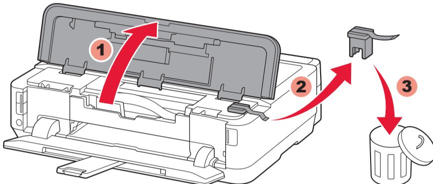
**2** Open the Top Cover. Remove the orange tape and protective material.
