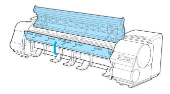
Grasp the Belt, insert it between the Belt Stopper, and affix the Belt Stopper with a hex screw at the position indicated.
