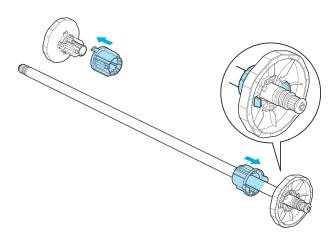
Insert the paper core, which serves as the spindle for rewinding a roll, on the Rewind Spool.
