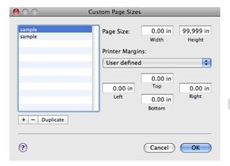
In Page Size, enter the height and width of the original. Here, enter 43.00 cm in Height and Width.
