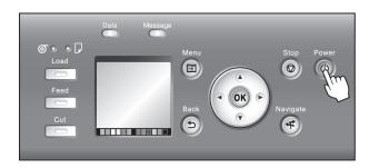
The **Power Lamp** is lit when the printer finishes starting up, and the printer is now in **Standby**.
