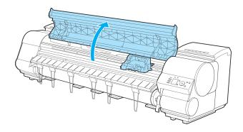
If the Cutter Unit or Carriage Cover is dirty, use a damp cloth that you have wrung out completely to wipe it clean.
