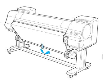
Making sure the roll paper is not slack, tape the left and right side of the leading edge to the paper core.
