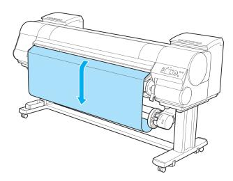
On the Right Media Take-up Unit, pull the Rewind Mode Switch forward to turn it on. Press the ▼ button to rewind the roll so that it is nearly taut.
