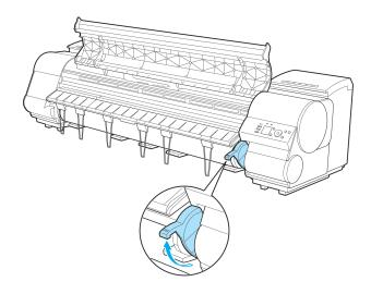
Hold the edge of the roll paper as you gently pull it evenly with both hands to the position of the Ejection Guide (a). Align the right side of the roll paper with the Paper Alignment Line (b), keeping this side parallel to the line, and then lower the Release Lever.
