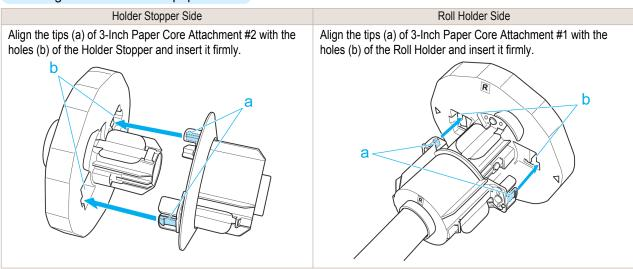
With the edge of the roll paper facing forward as shown, insert the Roll Holder from the right of the roll. Insert it firmly until the roll touches the flange (a) of the Roll Holder, leaving no gap.
