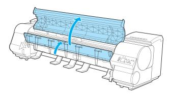
Remove the six Ejection Supports and lower the Ejection Guide.
