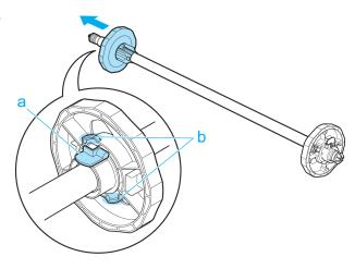
2 Insert the respective attachments for the roll paper core on the Roll Holder and Holder Stopper.
