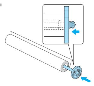
Load the roll in the printer. (See "Loading Rolls in the Printer.") P.485
