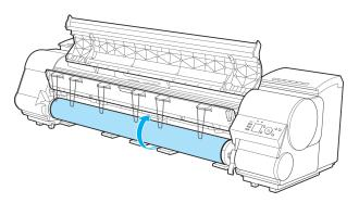
Holding the Roll Holder flange (a), remove the holder from the Roll Holder Slot.
