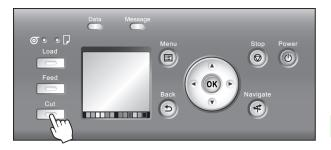
Press ▲ or ▼ to select **Yes**, and then press the **OK** button. After the roll paper is cut, it is rewound automatically.
