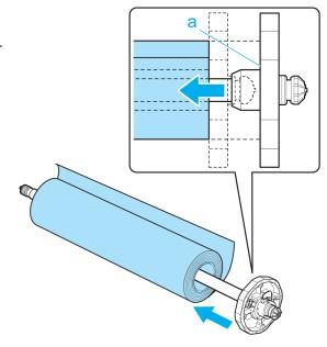
Insert the Holder Stopper from the left in the Roll Holder as shown. Holding it at the position shown (b), push it firmly in until the flange (a) of the Holder Stopper touches the roll. Lock the Holder Stopper lever (c) by pushing it down toward the shaft side.
