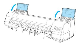
2 Lift the stopper (a) of the lnk Tank Lock Lever (a). Lift the lnk Tank Lock Lever until it stops, and then push it down to the front.
