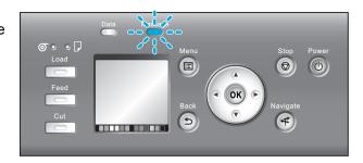
If the **Data Lamp** is flashing, the printer is receiving a print job. Turn off the printer only after printing is finished.
