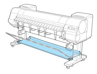
Remove the Output Stacker from the printer.
