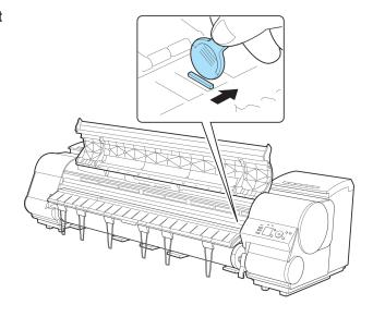
Refer to the following table to confirm the number on the Platen (a) that corresponds to the size of paper for printing.
