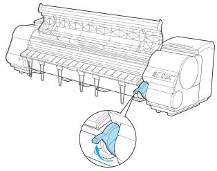
5 Keeping the right edge of the paper aligned with the extended line of the paper alignment line (a) on the right side of the printer and the position from which to start printing aligned with the groove (b) at the far end of the platen, load the paper.
