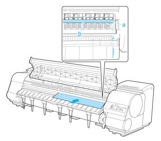
**6** Lower the Release Lever and close the Top Cover.
