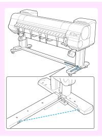
Unlock the flange on the left side of the Rewind Spool by lifting the lever (a) from the shaft side. Remove the flange.
