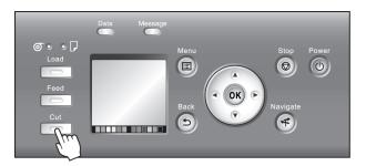
Press ▲ or ▼ to select **Yes**. As you hold the trailing edge of the printed document, press the **OK** button. The roll is now cut.
