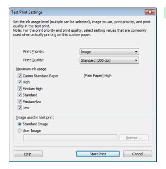
12 Determine and set the ink level that is thought to give the best visual test print results with no bleeding or scraping of ink.
