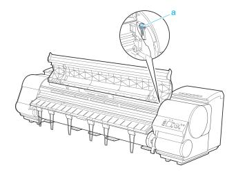
**4** Using the back of the Cleaning Brush, move the first Switch to the side opposite ●.
