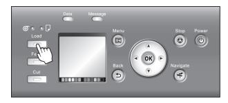
2. Press ▲ or ▼ to select Load Cut Sheet, and then press the OK button.
