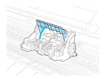
5 Pull the Printhead Fixer Lever forward all the way to open it completely.
