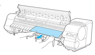
If the paper is not visible, lift the Ejection Guide, remove the Roll Holder, and clear the paper jam from below.
