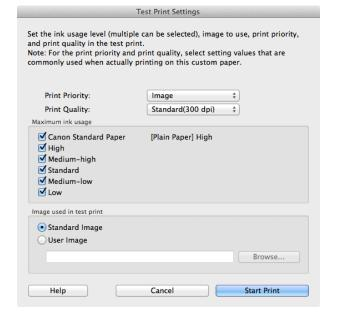
12 Determine and set the ink level that is thought to give the best visual test print results with no bleeding or scraping of ink.
