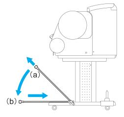
Remove the front Basket Rod from the left and right basket arms. Roll up the Basket Cloth and put it at the back of the Bottom Stand Stay.
