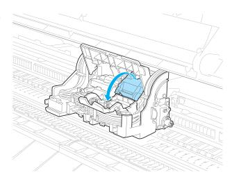
Push the Printhead Fixer Lever toward the back of the printer until it clicks.
