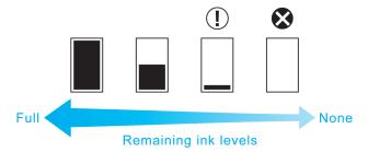
If the Display Screen indicates to replace the lnk Tank, replace the lnk Tank. If a message is displayed indicating to check the remaining ink levels, or after tasks that consume a lot of ink such as large-format printing or head cleaning, check the remaining levels and replace lnk Tank as needed. (See "Replacing lnk Tanks.") —P.758
