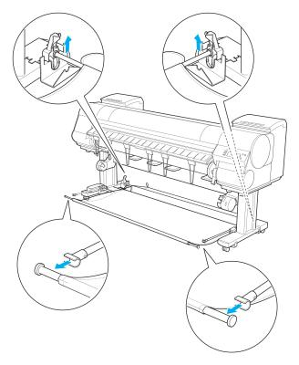
3 Stow the left and right basket arms. Next, with the Rod Holder still attached, remove the Rod Holder Adapter and put it in front of the printer.
