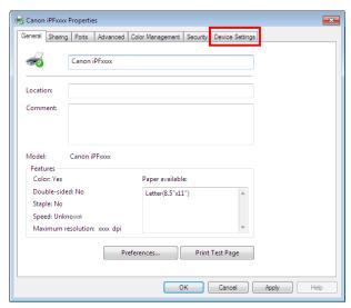
Device Settings Sheet →P.189 You can display settings for optional equipment installed on the printer and see the version information for the printer driver.
