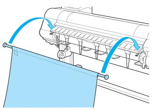
Form the Basket Cloth into a sloping shape to make it taut, and attach the middle Basket Rod to the Rod Holder.
