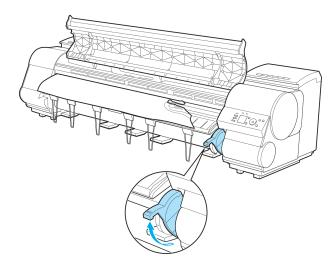
Holding the paper on both sides, pull the jammed portion out toward the front. Use scissors or a cutting tool to cut away the printed or wrinkled portion.
