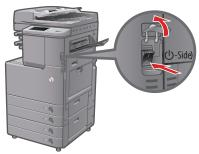
However, for the imageRUNNER ADVANCE, you just need to open the main power switch cover located on the right side of the machine, and push the main power switch toward the "O" side.
