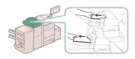
Remove any paper jammed in the upper cover (I-I1) of the document insertion unit.
