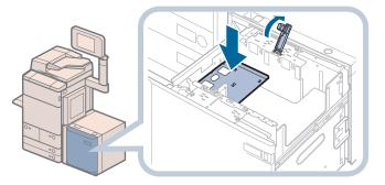
If you are not using the deck base plate, move the POD Deck Lite-A1 away from the main unit, and hang it on the hook that is on the inner left side of the POD Deck Lite-A1.
