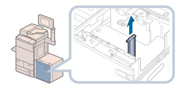
Remove the two blue screws on the outer size change plate using a coin or something similar.
