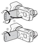
Open the LCD panel and adjust the angle.
