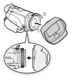
Place the lens hood on the front of the lens so that the groove on the lens hood is aligned with the bottom of the lens (①), and then turn the lens hood clockwise until it stops with a click (②).
