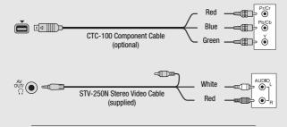
3 Composite video connection: Analog, standard-definition connection.
