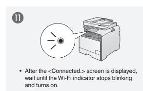
Wait approximately 2 minutes after the connection is completed. The IP address is set during this time period.
