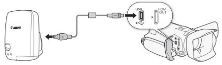
When connecting the GP-E2 GPS Receiver to the camcorder, use the connecting cable supplied with the receiver.
