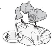
2 Firmly tighten the front and rear screws with a coin or similar object.
