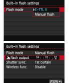
Normally, set this to [**E-TTL II**]. This enables autoexposure shooting with the built-in flash.
