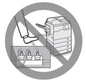
The power cord should not be taut, as this may lead to a loose connection and cause overheating, which could result in a fire.
