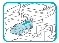
Insert the toner cartridge into the machine as far as it will go.
