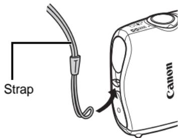
If you put the camera in the Waterproof Case without first removing the strap, the strap may catch in the waterproof seal when opening or closing the Waterproof Case. This can cause leaks.
