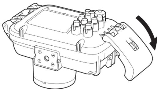
**7** Turn the mode dial in the direction of the arrow to engage the camera's mode dial.
