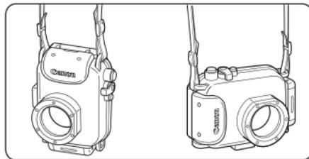
Use the neck strap when carrying the camera on the beach. Remove the neck strap and attach the wrist strap before use underwater. There is danger that the neck strap will become entangled and cause strangulation or another mishap.
