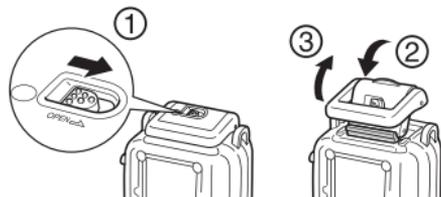
Apply a thin coat of grease to the entire seal before using the Waterproof Case in order to prevent abrasion and deterioration. For waterproof seal handling precautions, see *Waterproof Seal* (p 6).
