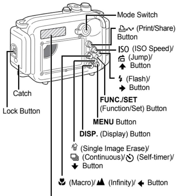
Apply the included controls layout sticker to this area to aid in using the camera controls.
