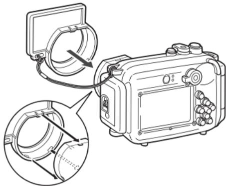
**Be sure not to trap the cord of the diffusion plate when closing the catch of the Waterproof Case.**
