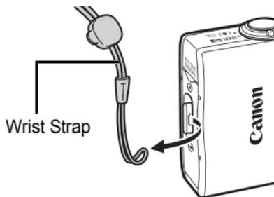
The camera's strap may catch in the waterproof seal when opening or closing the Waterproof Case and cause leaks if it is not removed.
