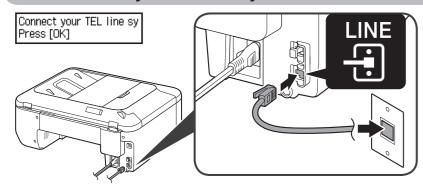
Connect the machine to a telephone jack with the supplied telephone line cable. then press the **OK** button
