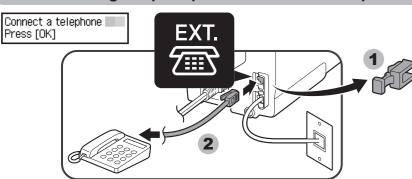
If you want to connect a telephone or an answering machine, remove the Cap, connect a telephone or an answering machine with a telephone line cable and press the **OK** button.
