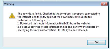
If this message is displayed, the media information file could not be downloaded automatically from the Internet. Configure the settings using the following procedure.
