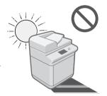
Avoid locations where a considerable amount of dust accumulates./Avoid locations near volatile or flammable materials, such as alcohol or paint thinner./Avoid locations where ammonia gas is emitted.
