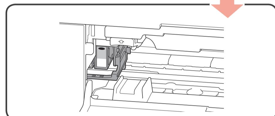
An installed ink tank cannot be removed until the message to replace it is displayed.
