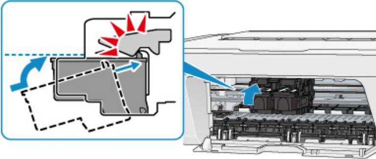
After confirming that the FINE cartridge is installed properly, close the cover.
