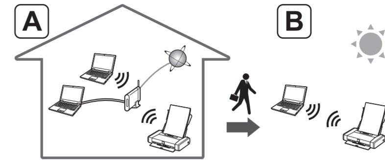
If you usually use the printer via a wireless router and want to use it without the router, change the connection method to the direct connection. For information about changing the connection method, refer to the Online Manual below.
