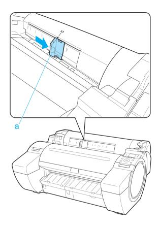
Load a single sheet printing-side up in the Paper Feed Slot, with the right edge aligned with the Paper Palignment Guide (a) to the right of the Roll Cover.
