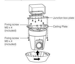
Use the junction box plate (included with the ceiling mount cover (sold separately)) to mount the camera to the junction box. ① Attach the junction box plate to the junction box with screws that match the screw holes in the junction box.
