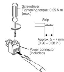
12 V DC can be connected in a non-polar configuration.
