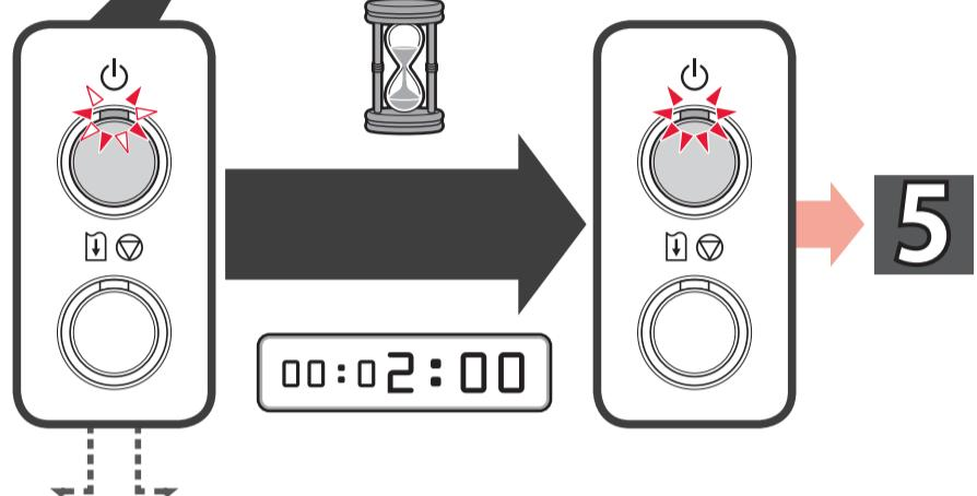
If the **Alarm** lamp flashes, check that the Print Head and ink tanks are installed correctly.
