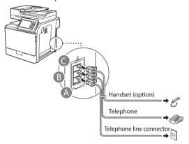
When <Connect Telephone Line> appears on the display, connect the telephone cable by referring to the illustration.
