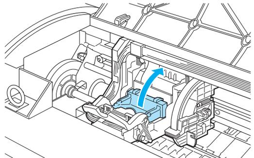
**5** Remove the Printhead and press the **OK** button.
