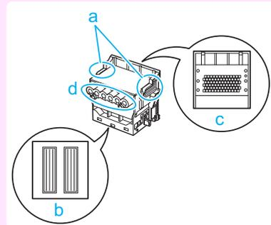
**7** While firmly holding the Printhead you have removed, use your other hand to remove the orange Protective Part (a). Squeeze the grips (c) of Protective Part (b) and pull it down to remove it.
