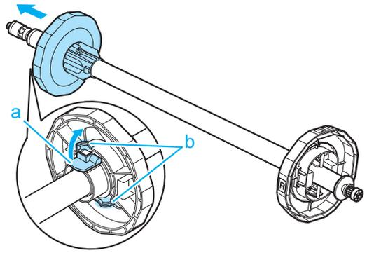
**2** Insert the respective attachments for the roll paper core on the Roll Holder and Holder Stopper.
