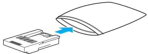
**5** Confirm the Maintenance Cartridge is right-side up, put it in the box with the packaging material attached, and store it so that it stays level.
