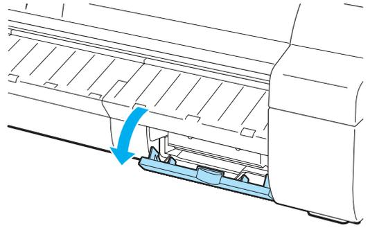
**3** Hold the used Maintenance Cartridge by the grip (a) with one hand and put your other hand under the Maintenance Cartridge to hold it firmly on the bottom, keeping it level as you pull it out.
